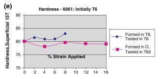
**Fig. 1** (a) Ultimate strength of the 6061 alloy initially in the T6 condition (b) Yield strength of the 6061 alloy initially in the T6 condition (c) % Elongation of the 6061 alloy initially in the T6 condition (d) Conductivity of the 6061 alloy initially in the T6 condition (e) Hardness of the 6061 alloy initially in the T6 condition
