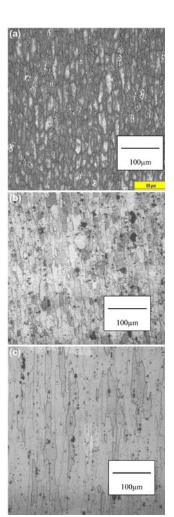
**Fig. 4** (a) 6061 Stretched 16% in O, Heat treated to T62: Longitudinal view  $(200 \times)$  (b) 2024 Stretched 4% in O, Heat treated to T62: Longitudinal view  $(200 \times)$  (c) 7075 Stretched 6% in O, Heat treated to T62: Longitudinal view  $(200 \times)$
