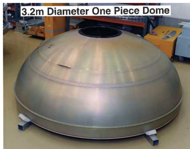
Fig. 1 One-piece dome for a cryogenic tank (2219 alloy)
