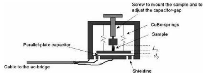
Fig. 3 Capacitance dilatometer for measuring material CTE
