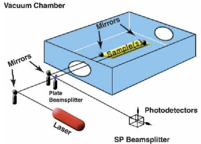
Fig. 2 Michelson laser interferometer for measuring material CTE
