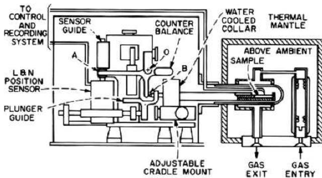
Fig. 1 Push-rod dilatometer for measuring material CTE
