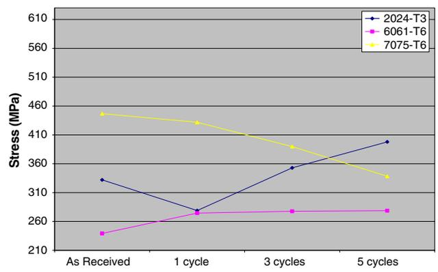
**Fig. 6** Yield strength for all alloys after high heat treatments, at 205 °C
