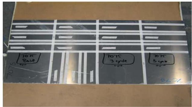
Fig. 3 Marked rectangular samples on uncoated sheet
