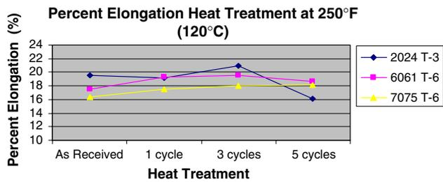
Fig. 13 Percent elongation for all alloys after low heat treatments
