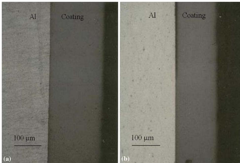
**Fig. 15** Coating thickness of 7075-T6 and 6061-T6: (a) 6061-T6, high-temperature cure, and (b) 7075-T6, high-temperature cure
