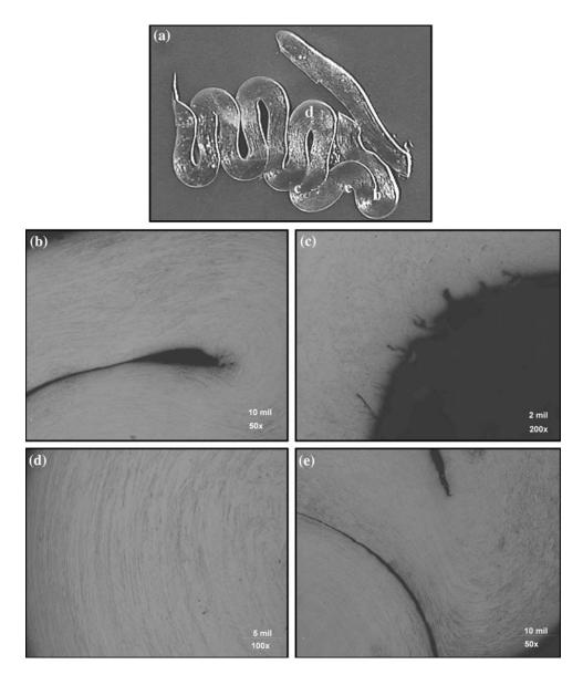
Fig. 11 (a) Copper sample biaxially crushed with a  $45^{\circ}$ . (b) Copper compressed microstructure ( $50\times$ ). (c) Microstructure shows evidence of flow lines and stress cracks ( $50\times$ ). (d) Copper microstructure bulk material flow lines ( $100\times$ ). (e) Compression area microstructure with stress cracks ( $200\times$ )
