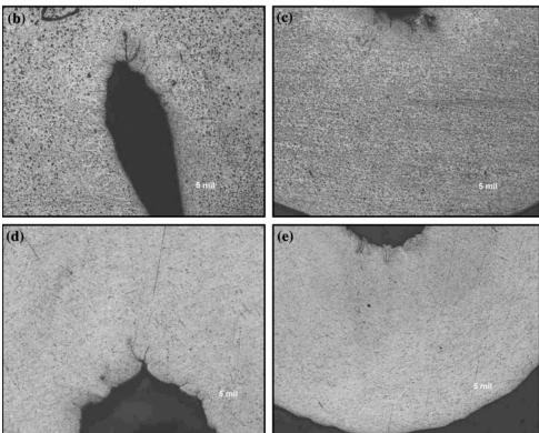
Fig. 5 (a) Aluminum sample biaxially buckled at a 45°. (b) Close up microstructure of the compressed portion of the aluminum crushed sample (50×). (c) Closed up microstructure of the bulk material of the aluminum crushed sample (50×). (d) Close up of the microstructure at the compressed portion of the aluminum crushed sample (50×). (e) Microstructure of the tension and compression portion of the crushed sample (50×).
