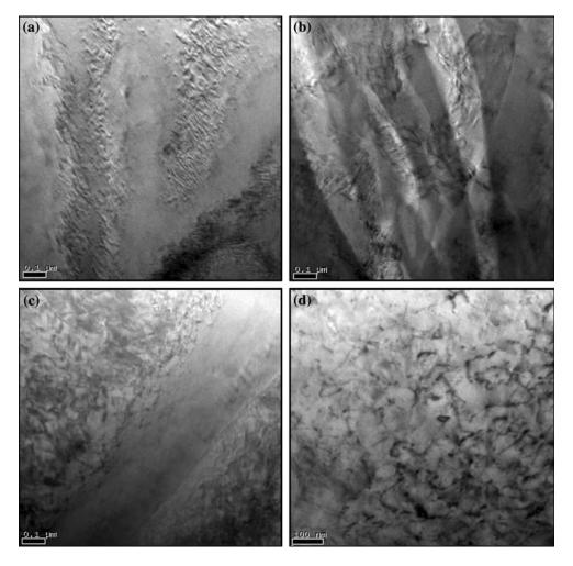
**Fig. 6** (a) TEM image of uniaxial deformed aluminum alloy tube, with dislocation cell structures. (b) TEM image of uniaxial deformed aluminum alloy tube with deformation bands. (c) TEM image of biaxial deformed (-45°) aluminum alloy with evidence of deformation bands. (d) TEM image of biaxial deformed (-45°) containing a cellular structure
