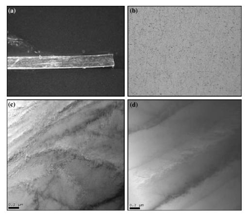
Fig. 3 (a) As-received aluminum with no buckling (b) As-received aluminum with no buckling (200×). (c) As-Received TEM image of the microstructure demonstrating dislocation cell structure and sub-structure. (d) As-Received TEM image of the microstructure with evidence of oriented textured structure
