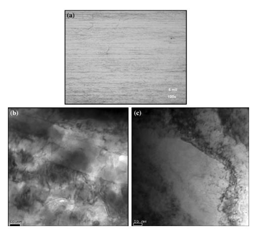
Fig. 7 (a) As-Received Copper sample with material flow lines (100×). (b) TEM image of as-received copper tube with textured structure and dislocation network. (c) TEM image of as-received copper tube with evidence of dislocation cells
