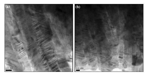
Fig. 13 (a) TEM image of biaxial deformed (-45°) copper tube: Deformation bands, Twins, and Slip bands. (b) TEM image of biaxial deformed (-45°) copper tube: Deformation bands, Twins, and Slip bands
