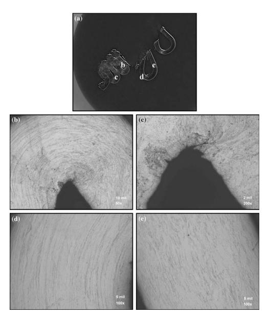
Fig. 9 (a) Biaxially buckled copper alloy sample at  $37^{\circ}$ . (b) Overall bend features (50×). (c) Compression stress cracks (200×). (d) Curved flow lines (100×). (e) Straightened flow lines (100×)
