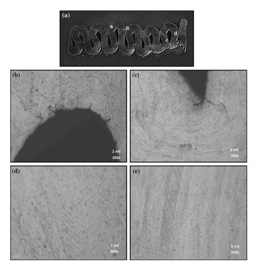
Fig. 8 (a) Biaxially buckled copper alloy sample at  $30^{\circ}$ . (b) Compression stress cracks ( $200\times$ ). (c) Compression stress cracks ( $100\times$ ). (d) Second-phase particles in the matrix ( $500\times$ ). (e) Another view of the second-phase particles in the matrix ( $200\times$ )
