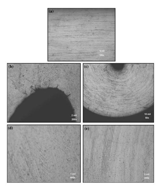
Fig. 10 (a) Biaxially buckled copper sample at  $30^{\circ}$  ( $100\times$ ). (b) Compression stress cracks ( $200\times$ ). (c) Tension and compression sides of the sample bend showing flow lines ( $50\times$ ). (d) Second-phase particles in the matrix ( $500\times$ ). (e) Another view of the second-phase particles in the matrix ( $200\times$ ).
