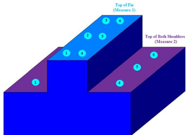
Fig. 4 Location of 18 different points measured on each “T” section. Six additional measurements were taken on the bottom side of the sample (measure 3)
