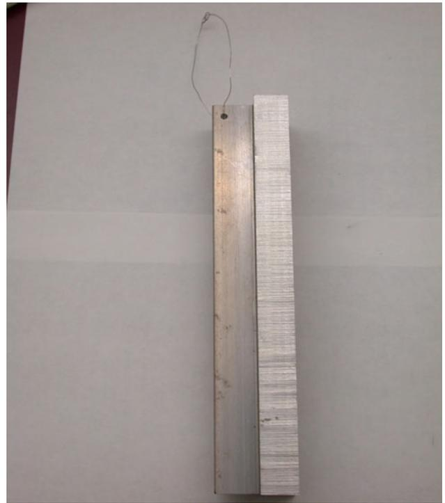
Fig. 3 Initial T section with hole and wire for quenching
