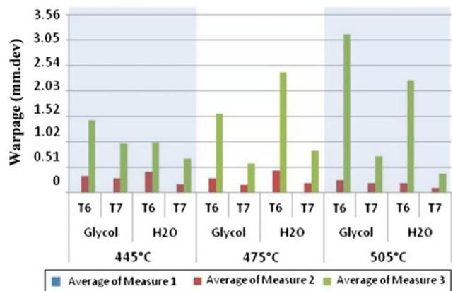
Fig. 11 T6 phase vs. T7' phase for cut 3
