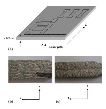
**Fig. 2** (a) Schematic view of a laser-formed Ti-6Al-4V plate from which tensile samples were extracted. The *dotted lines* depict the path of metal deposition. The actual plates were approximately 0.2 cm (0.08 in.) thick. (b) As-deposited surface in the *x-direction*. The specimen is 0.9525 cm (0.375 in.) wide. (c) As-deposited surface in the *z-direction*. The specimen is 0.9525 cm (0.375 in.) wide
