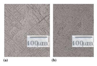
Fig. 7 Long (a) and rolling (b) direction views of the wrought Ti-6Al-4V microstructure after being annealed (beta-aged) at 865 °C
