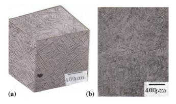
**Fig. 8** (a) An isometric view of the microstructure of the as-deposited sample. (b) A longitudinal view of the microstructure of the as-deposited sample
