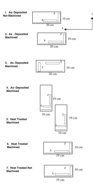
Fig. 3 Schematic views of the orientations of the tensile samples. This figure is intended to display the nomenclature used in this article
