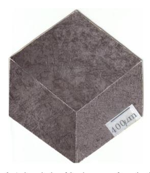
Fig. 9 An isometric view of the microstructure of an as-deposited machined sample
