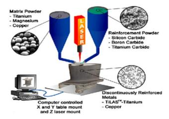
Fig. 1 Schematic view of laser forming
