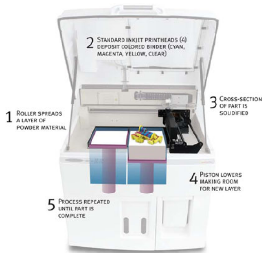
Fig. 2 Diagram of how the Spectrum Z510 Full Color System works (Ref 5)
