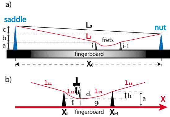
Fig. 2. Geometrical deformation model of a guitar string. (a) Original string (of length  $L_0$ ) and the deformed string (of length  $L_i$ ) when it is pressed between frets  $i$  and  $i-1$ . (b) The deformation model in terms of the four different sublengths  $l_{i1}-l_{i4}$  of the deformed string.
