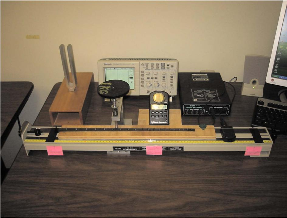
Fig. 3. Experimental apparatus composed of a standard sonometer to which we added a classical guitar fingerboard, visible as a thin black object with 20 metallic frets glued to a wooden board to raise it almost to the level of the string. Also shown is a mechanical device used to press the string on the fingerboard and several different instruments used to measure sound frequencies. This digital tuner is shown near the center, just behind the sonometer.
