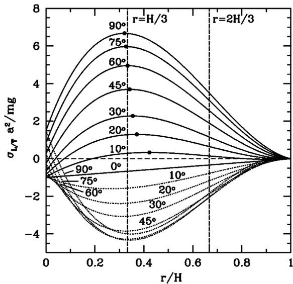
Fig. 6. The normalized longitudinal stress at the leading edge (solid line) and at the trailing edge (dotted line), are shown as a function of the height fraction and for several angles ( $H/a=24$ ). The maxima of the leading edge stress curves are marked by solid points.
