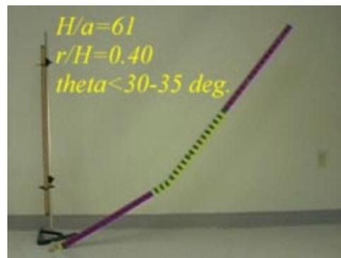
Fig. 9. The second toy model made with plastic blocks. The structure appears to break at  $r/H = 0.40$ , and at a larger angle  $\theta \approx 30^\circ - 35^\circ$ , which can be estimated by measuring the angle formed by the upper part of the tower with the vertical.
