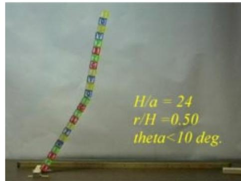
Fig. 8. The first toy model made with wooden blocks. The structure appears to break at  $r/H = 0.5$ , and at a small angle  $\theta \approx 10^\circ$ , which can be estimated by measuring the angle formed by the upper part of the tower with the vertical.
