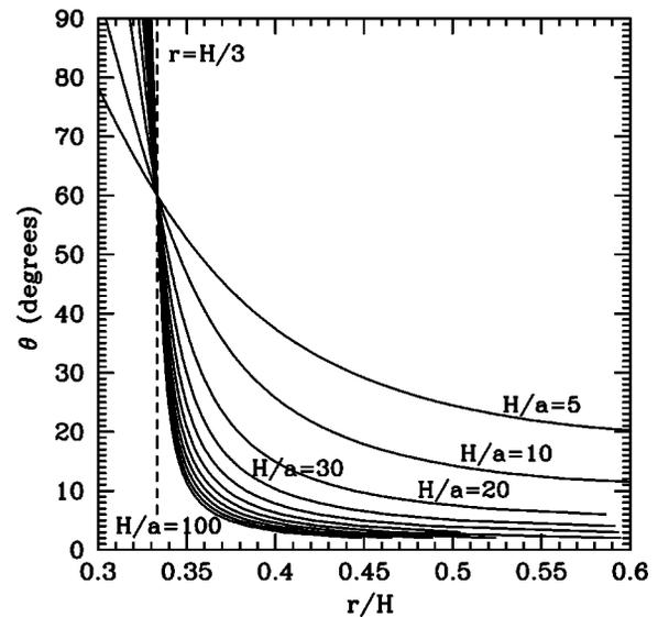
Fig. 7. The maxima of the leading edge stress curves are shown as continuous functions, for several values of the ratio  $H/a$ . They represent the points, in terms of the height ratio  $r/H$  and angle  $\theta$ , at which the structure is more likely to break, due to bending.
