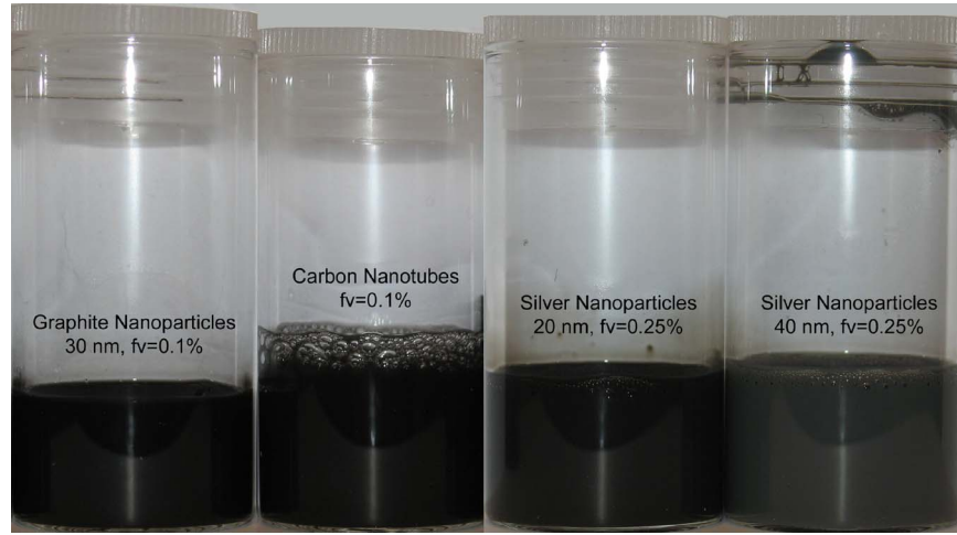
FIG. 2. Representative nanofluid samples tested in microcollector.
