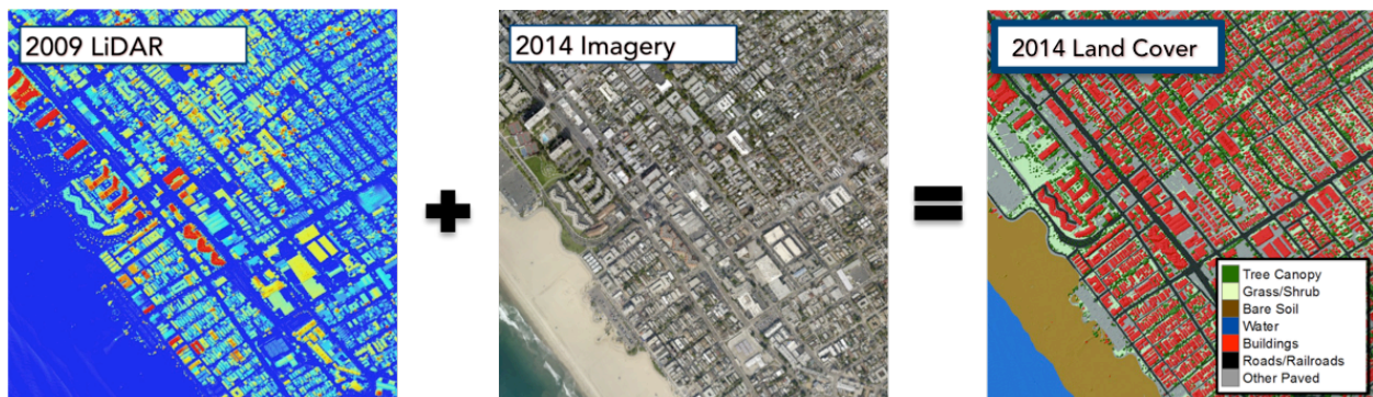
Figure 37. Land cover analysis combined 2009 LiDAR data and 2014 spatial imagery to produce a seven-category land cover classification map.
