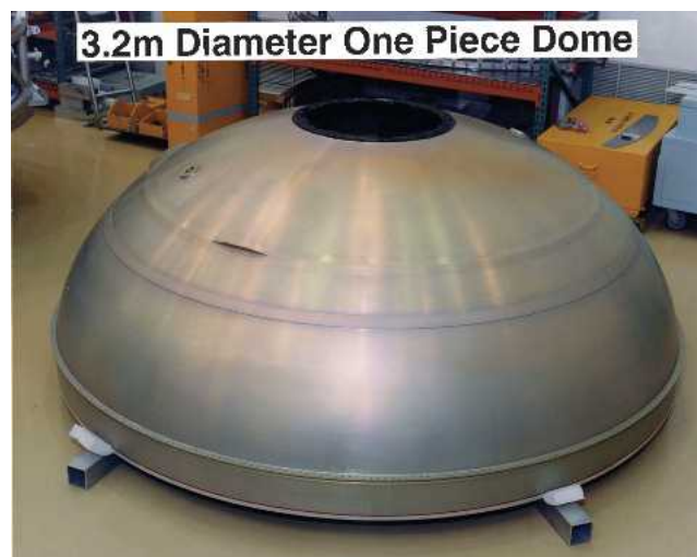
Fig. 1 One-piece dome for a cryogenic tank (2219 alloy)
