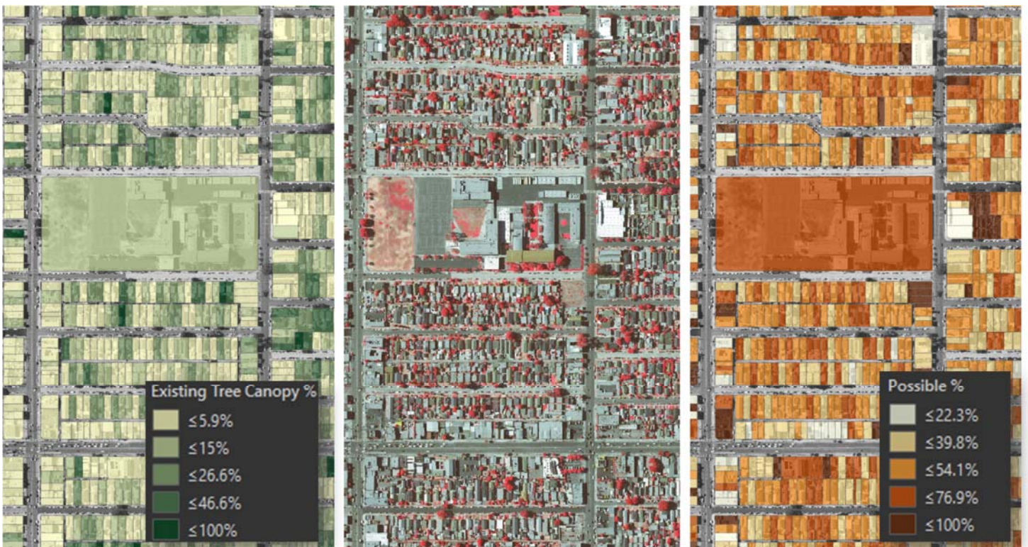
Figure 4: An example of tree canopy metrics computed at the property parcel level.
