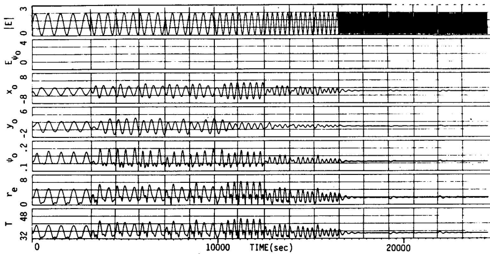
Fig. 11 Regular records, D-32% T_{BR} —BF6, fairleads at circumference
