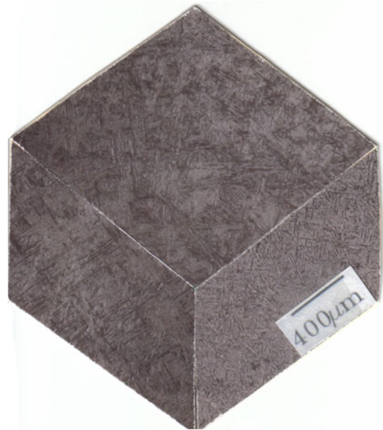
Fig. 9 An isometric view of the microstructure of an as-deposited machined sample
