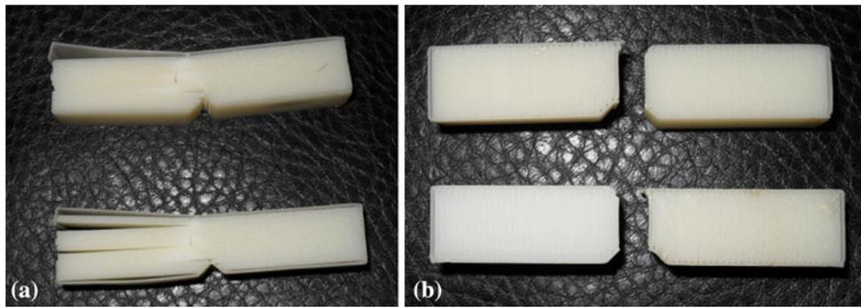
**Fig. 14** Izod impact test samples from Es-Said et al. (a) arrestor/0° and (b) transverse/90°
