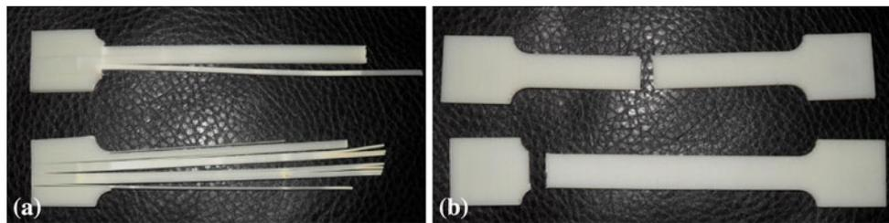
**Fig. 13** Tensile test samples from Es-Said et al. (a) arrester/0° and (b) transverse/90°
