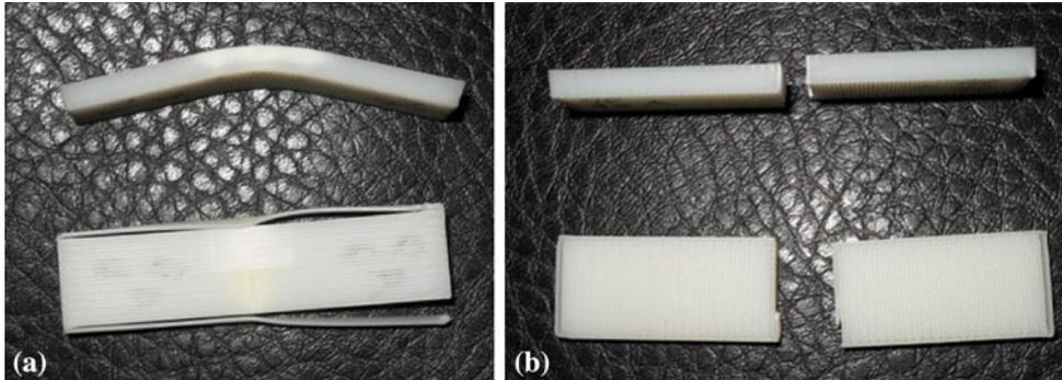
**Fig. 15** Three-point bend test samples from Es-Said et al. (a) arrestor/0° and (b) transverse/90°
