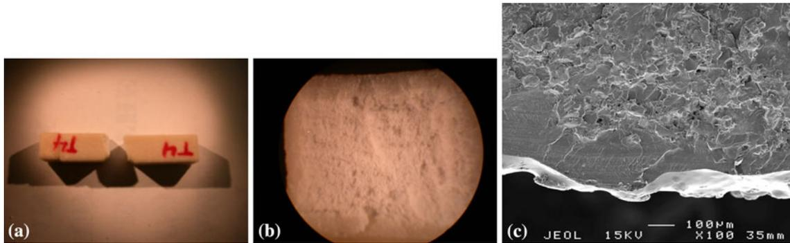
**Fig. 12** Photo documentation of the Short Transverse (T) after Izod impact testing
