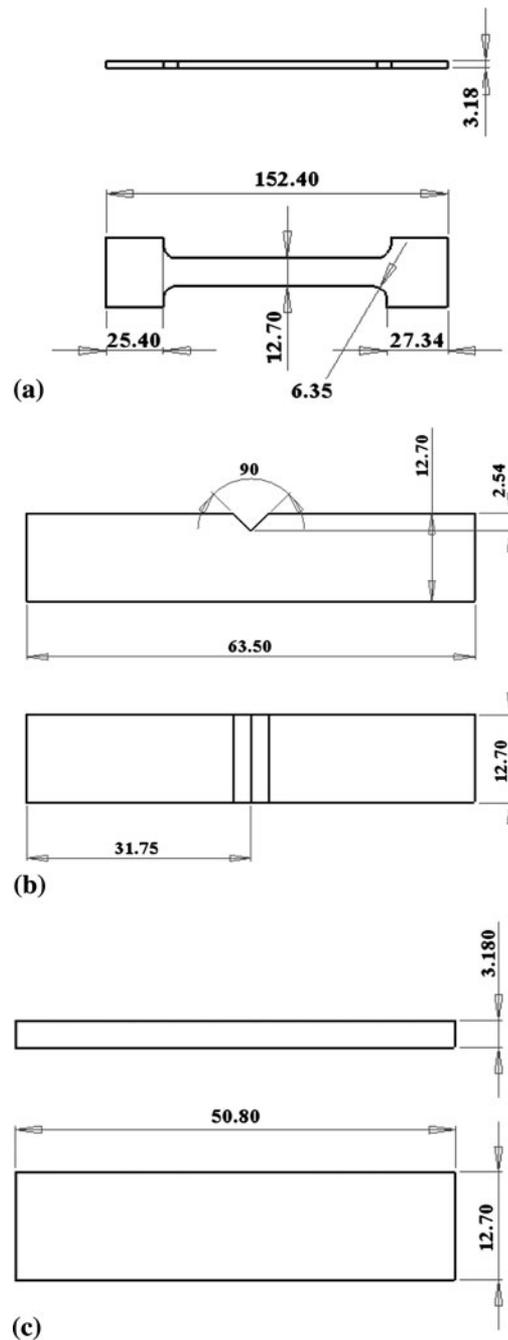
Fig. 3 Test sample dimensions (mm). (a) Tensile test sample dimensions, (b) Izod impact energy test sample dimensions, and (c) three-point bend test sample dimensions
