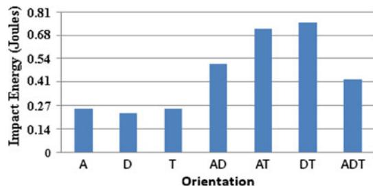
Fig. 6 Average impact energy values for Izod impact testing (J)
