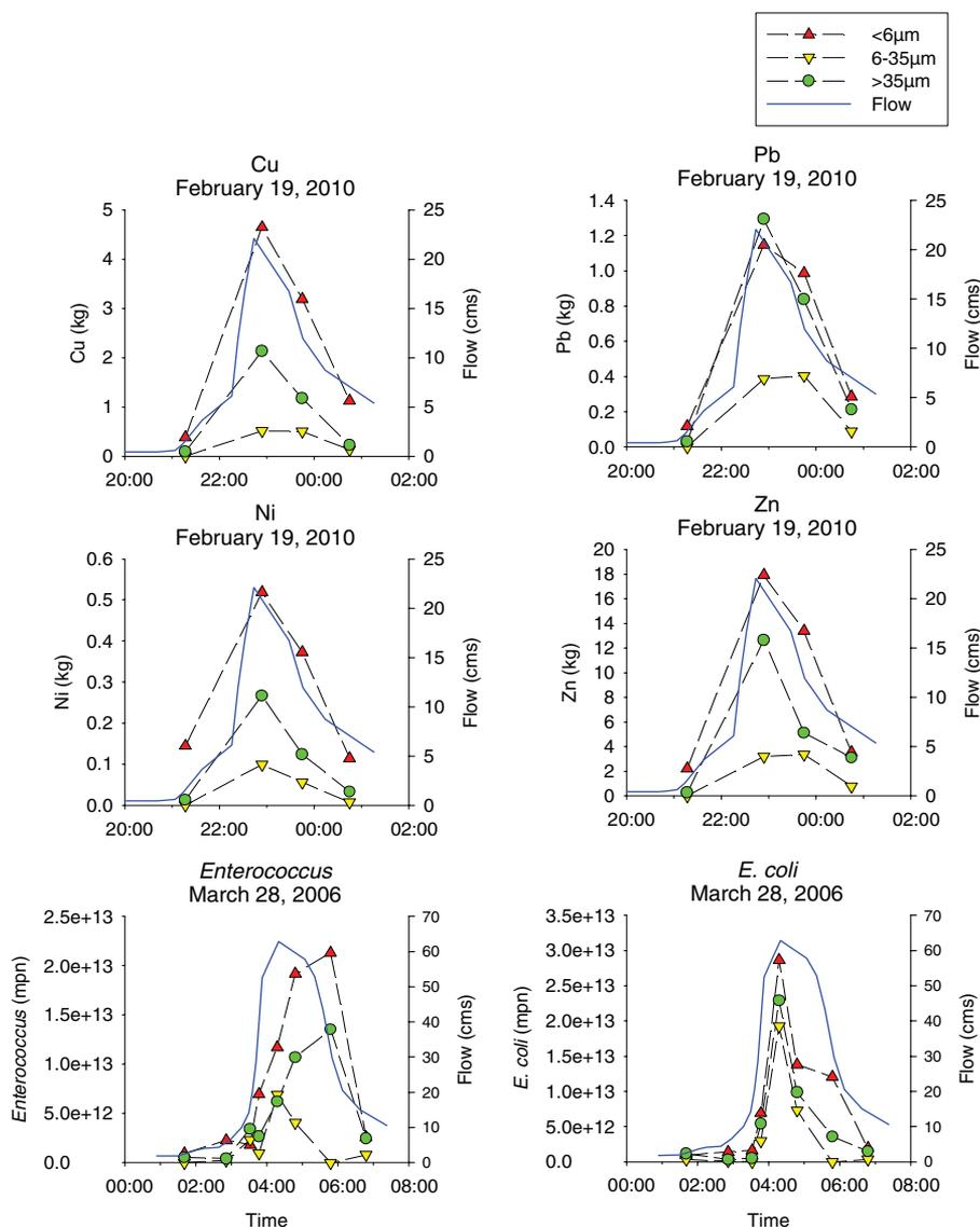
Fig. 4. Metal and bacteria mass discharge distributed among the three filter fractions, relative to storm flow rate. [Color figure can be viewed in the online issue, which is available at [wileyonlinelibrary.com](http://wileyonlinelibrary.com).]
