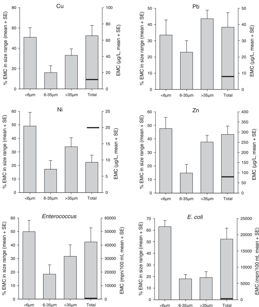
Fig. 2. Proportion of flow-weighted event mean concentration (EMC) associated with the various filter fractions (first three bars in each graph), and the overall EMC (fourth bar). The data represent the mean of the EMCs from the four (metals) or eight (bacteria) storm events. The vertical line above each bar represents the standard error (SE). The horizontal slash on the fourth bar indicates the water quality standard used for comparison.
