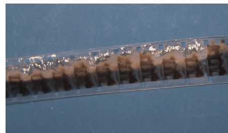
Fig. 21. Silver mirroring on 16 mm film
