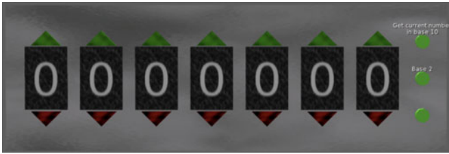
Fig. 1. HexWindow. Users controls whether to convert the number or use the window to count up/down as with an odometer.
