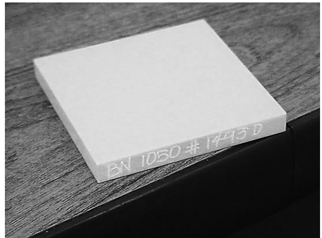
Fig. 4. One of the 17 different cortical bone phantoms from two sets, which varied in BMD from 0 to 1700 \text{ mg/cm}^3 .
