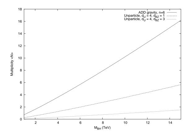
Figure 3: Comparison of ADD  $(M_D=1~{\rm TeV}, n=6)$  and unparticle-enhanced  $(\Lambda_{\mathcal{U}}=1~{\rm TeV}, M_{\mathcal{U}}=10~{\rm TeV}, d_{\mathcal{U}}=4, d_{\rm BZ}=1,3)$  decay multiplicities for LHC black holes for an integrated beam luminosity of 30 fb<sup>-1</sup>yr<sup>-1</sup>.
