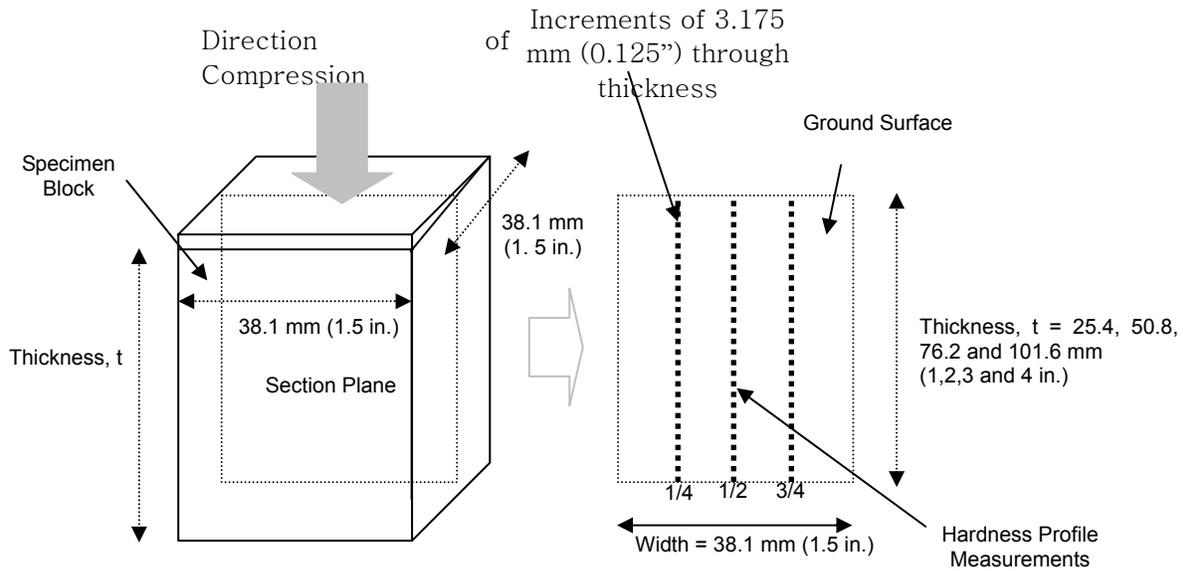
**Figure 2.** Specimen Configuration for Hardness Profiling
