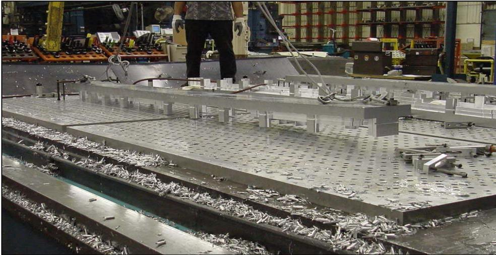
**Figure 1.** Distortion During Machining Due to Residual Stresses
