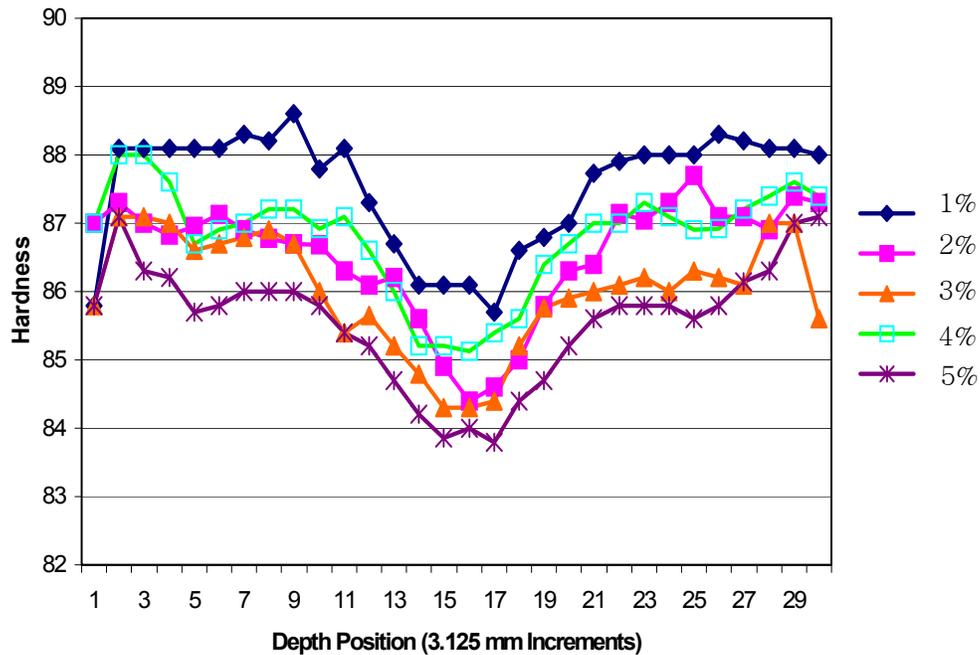
**Figure 6.** Hardness Profiles of 101.6 mm (4.0 in.) Sample Blocks as a Function of Compression
