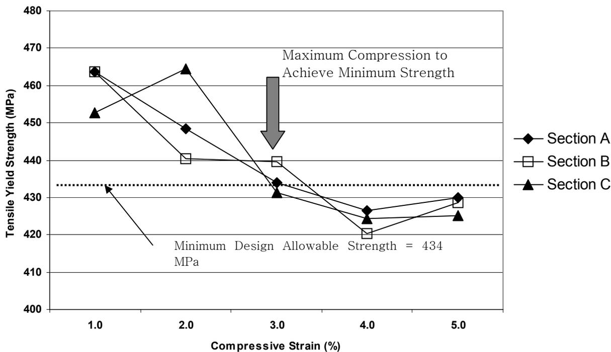
**Figure 7.** Effect of Compression on Tensile Strength After Aging
