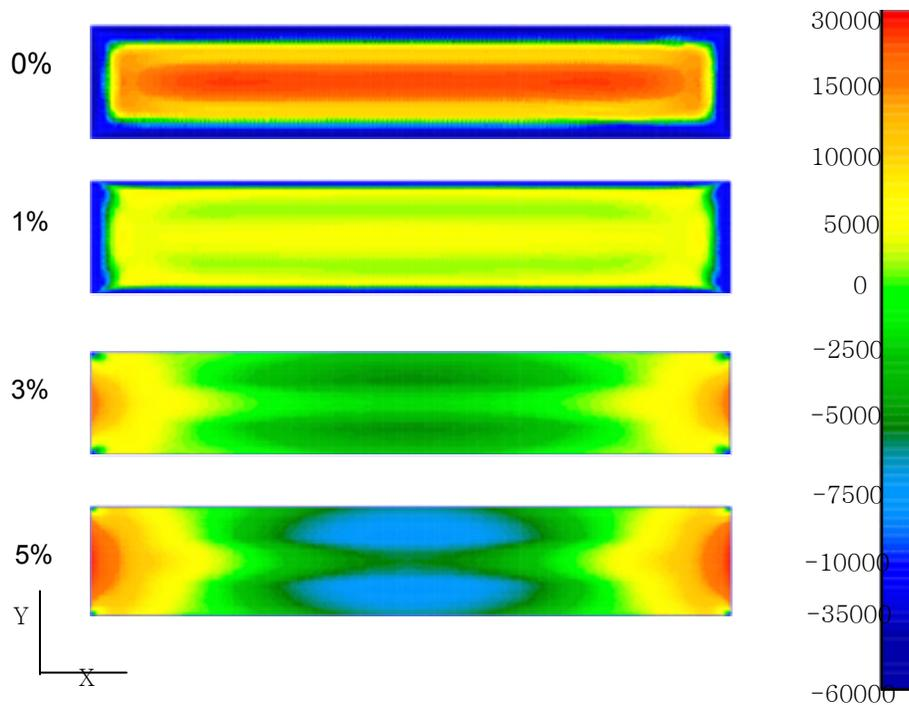
**Figure 8.** Residual Stress Profiles in Forged Billet as a Function of Compression Level as Predicted by Finite Element Analysis
