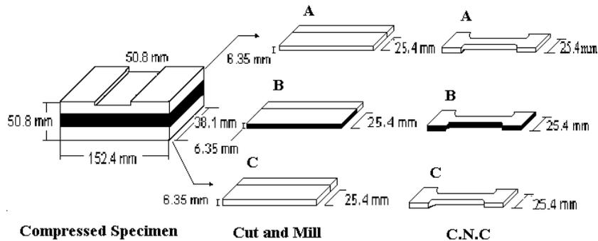
**Figure 3.** Specimen Configuration for Tensile Testing
