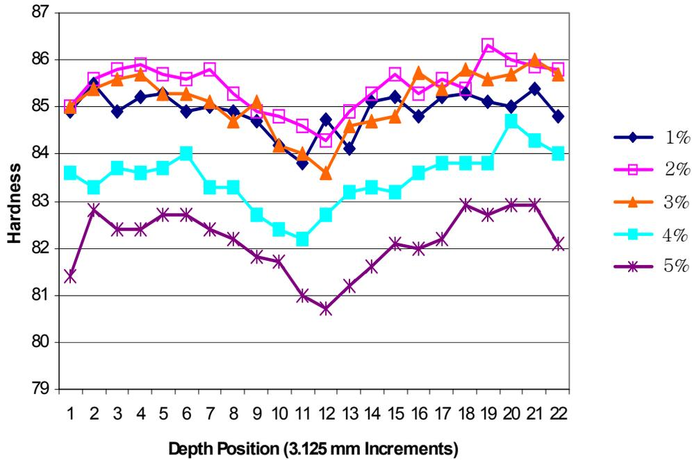
**Figure 5.** Hardness Profiles of 76.2 mm (3.0 in.) Sample Blocks as a Function of Compression
