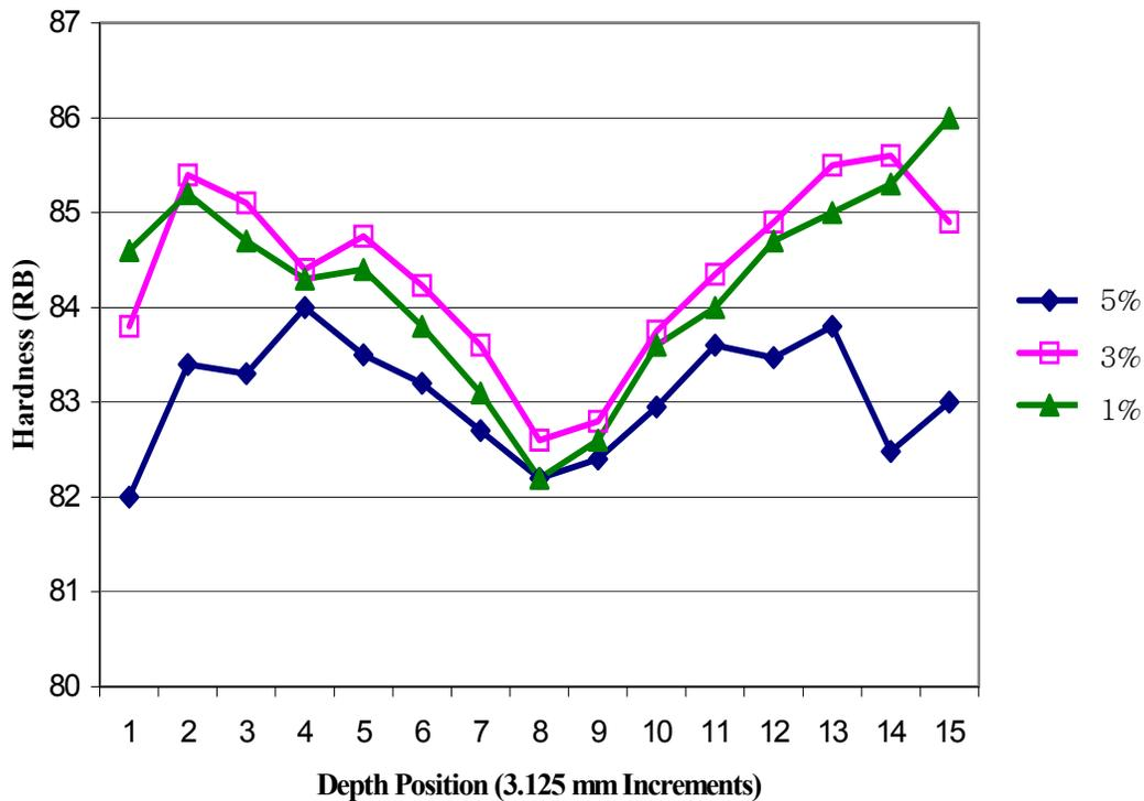
**Figure 4.** Hardness Profiles of 50.8 mm (2.0 in.) Sample Blocks as a Function of Compression
