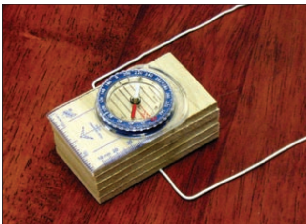
Fig. 1. Photograph of the U-shaped wire, compass, and wood spacers that are used to change the distance between the base segment of the wire and the compass.
