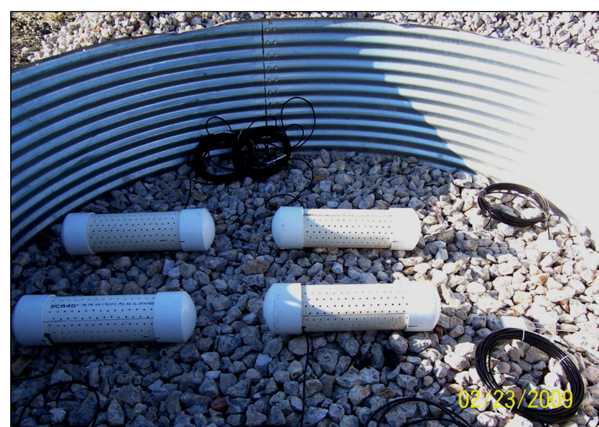
Figure 2. The response of TDRs in 1" diameter recycled concrete aggregate with protective PVC housing (left and center) and without housing (right) were studied at the pilot scale under unsaturated flow conditions.
