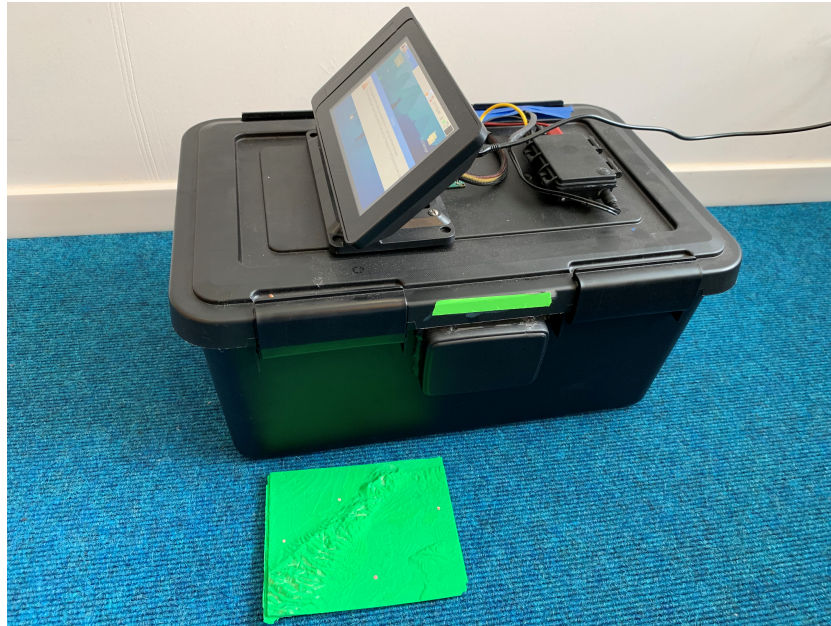
Figure 1 Photograph of the custom-designed and built Slime Mold Incubator Camera System (SMICS) used to capture the exploration of the slime mold over the 3D printed maps with one of the 12 cm x 15 cm maps included for scale.
