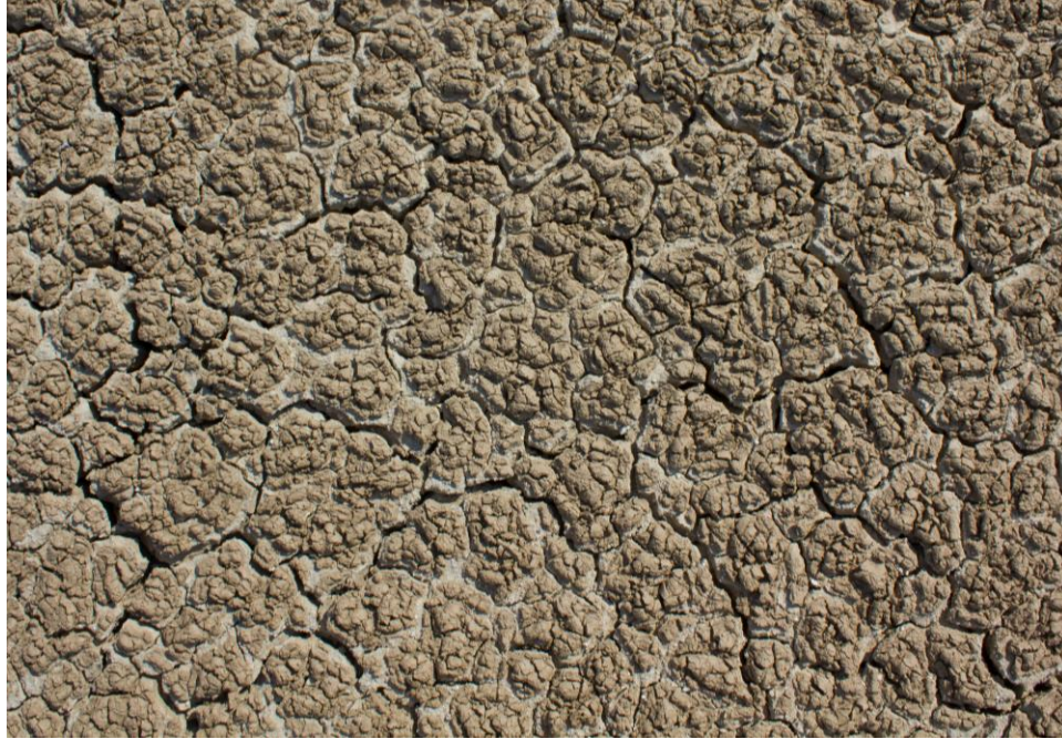
Figure 2: An image of the surface of RDL. Because of the high clay content, the soil shrinks and cracks if left dehydrated for an extended period.
