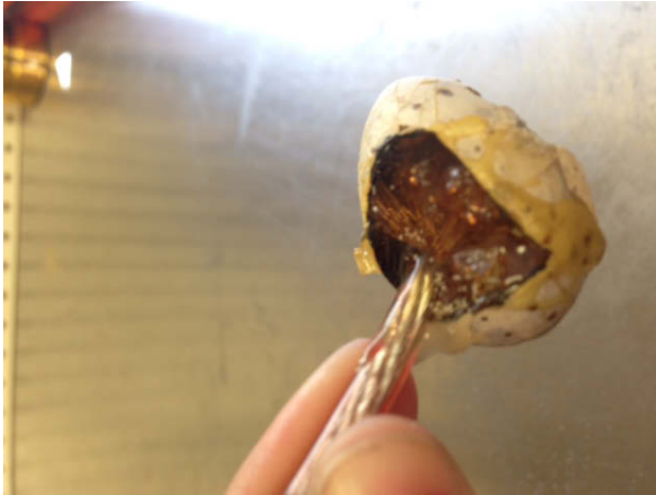
Figure 13: Underside of completed electrified egg. The egg contained an inner painting of conductive glue and was filled with copper mesh and epoxy glue, with speaker wire extending outward.
