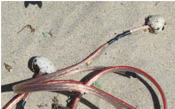
Figure 14: Two electrified eggs each connected to the network of speaker wires connecting all the electrified eggs to each other and the shocking unit. The connection of the electrified eggs to the network of speaker wires was soldered and covered with a heat shrink tube.
