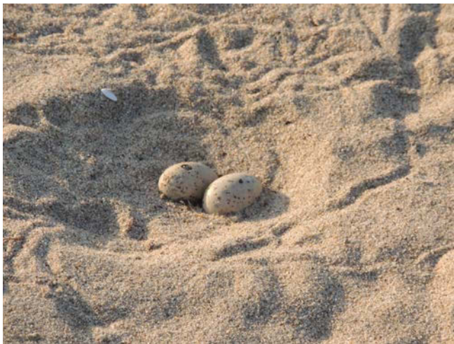
Figure 16: Pair of deployed electrified eggs within a depression in the sand to resemble a tern nest.
