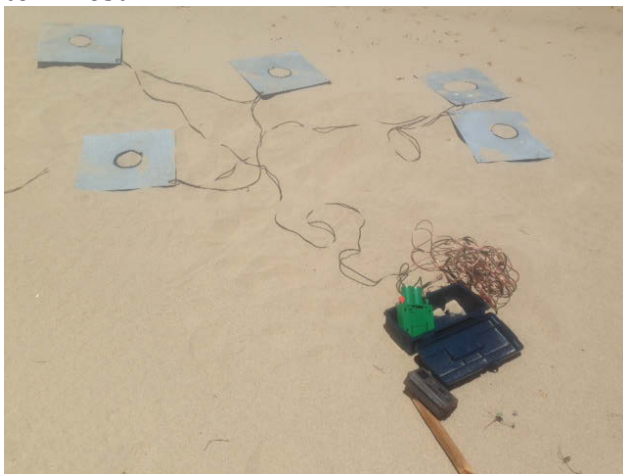
Figure 17: Steel plates and shocking unit with attached wires, laid on top of the sand prior to burying the items underneath the sand. The game camera fixed on the wooden stake laid on the sand prior to deployment.
