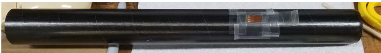
Figure 12: Carbon Fiber Reinforced Composite Tube Sample
