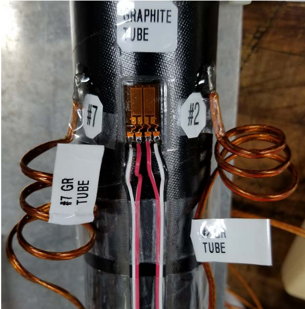
Figure 17: Completed Installation on Carbon Fiber Reinforced Composite Tube
