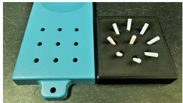
Figure 3. Modified Nine Hole Peg Test used in this study. The pegs begin in the board on the right. Each outside peg is oriented 30° outward from the center vertical peg. The time to move these 9 pegs, in any order, to the left board was recorded as the score.
