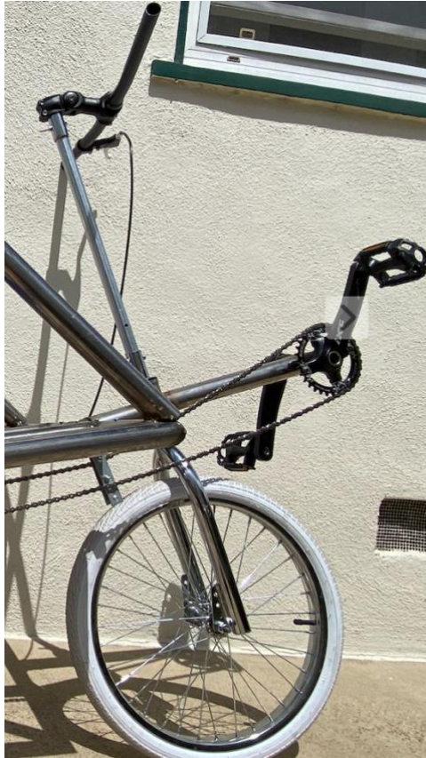
Figure 9: Steering and power generation shown with handlebars, fork, wheel, and pedals.
