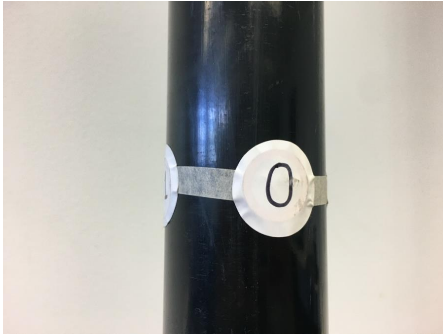
Fig. 34. Image demonstrating protrusion amount of RFID tags on the pole
