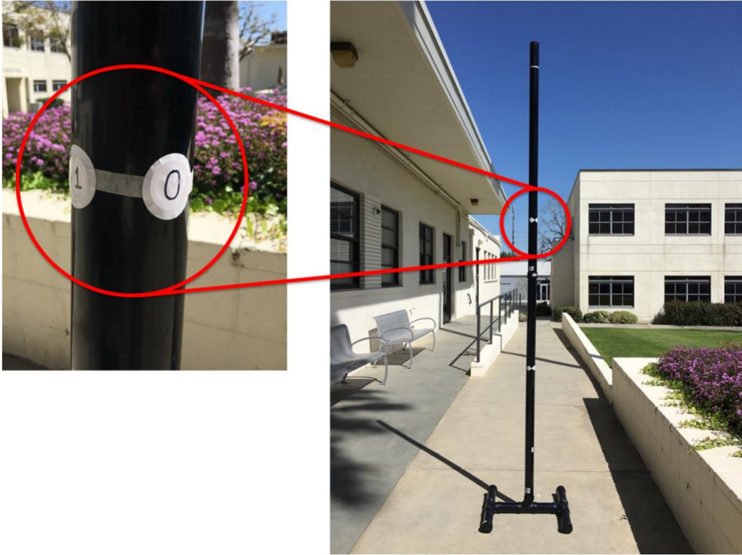
Fig. 23. Mock Chinese Pole constructed out of PVC pipes with RFID tag bands attached
