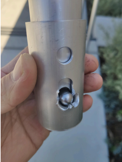
Figure 17- Compression Test: Aluminum Shaft Yielding
