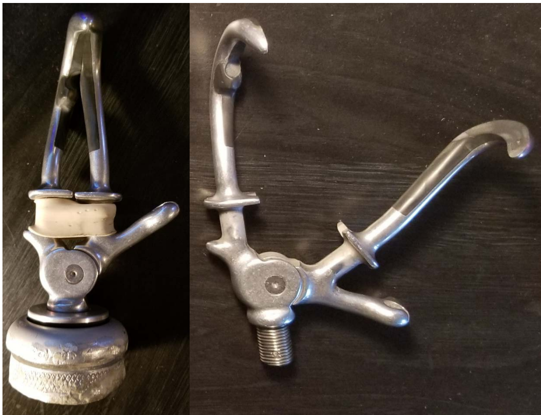
Figure 6: The Hosmer 5X Prosthetic Hook that was scanned and used for testing. This is a terminal device that is body powered operated. In the left image, the prosthetic hook is screwed in to the wrist attachment device.
