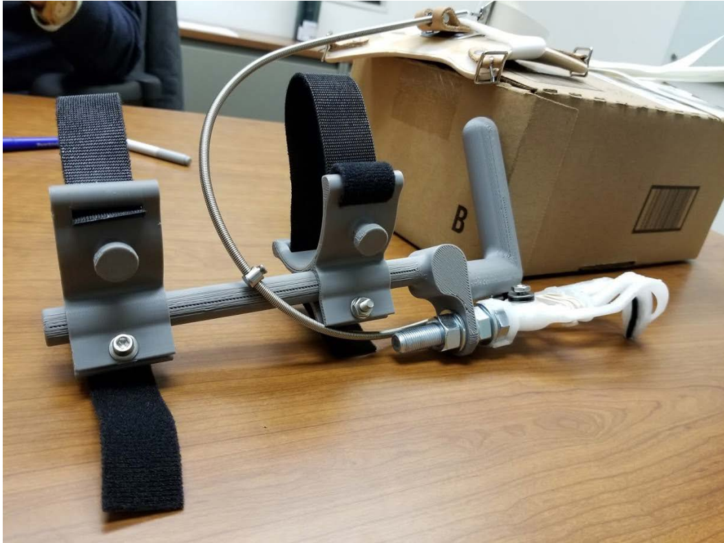
Figure 49: Simulator prototype number two with a sideways grabbing handle and round bar for the ribs to clasp on to.
