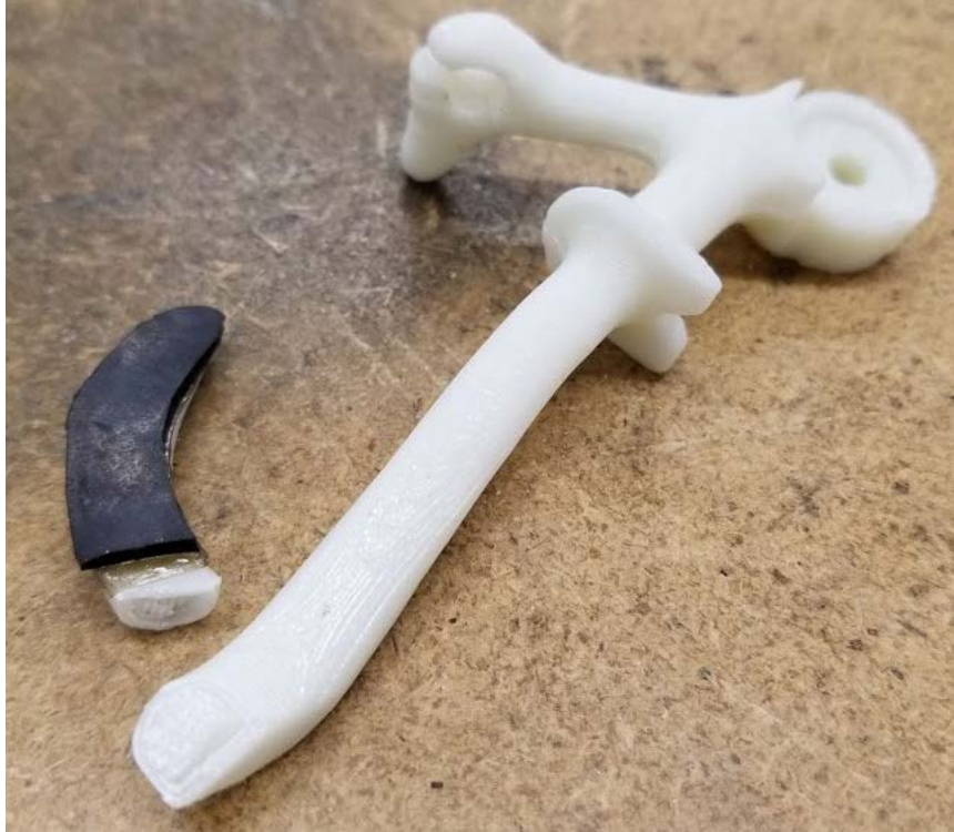
Figure 43: Post stress test of thumb half of the 3D printed prosthetic with no truss.
