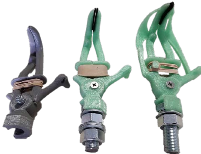
Figure 20: The first iteration of the 3D printed Hosmer 5X Prosthetic Hook (left, grey) and the final iteration of the Hosmer 5X Prosthetic Hook (right, green) with a M12-1.25 screw.
