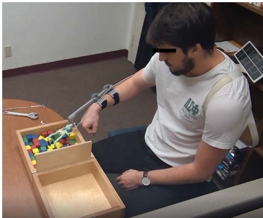
Figure 29: The Box and Blocks Test being performed with the above-arm simulator and the plastic prosthetic.
