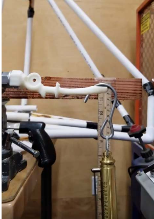
Figure 22: Stress test being performed on screw-housing side of the 3D printed prosthetic without the added truss.
