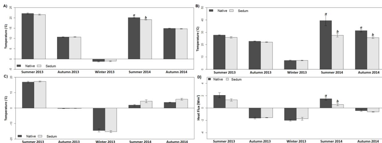
**Figure 4.** Average (A), maximum (B), and minimum (C) substrate temperature ( $^{\circ}\text{C}$ ) and average substrate heat flux  $\text{Wm}^2$  (D) at the NSCC green roof. Those bars that share a letter are not significantly different (within the same season).
