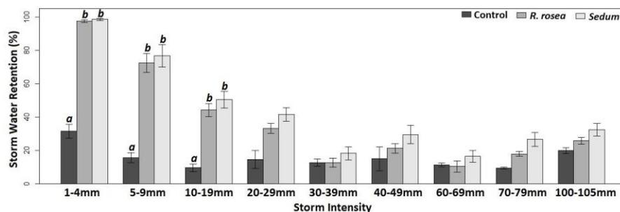
**Figure 6.** Average stormwater retention (%) for varying storm intensities at the SMU green roof for the conventional roof, the *R. rosea* treatment, and the *Sedum* treatment. Those bars that share a letter are not significantly different (within the same rainfall intensity).
