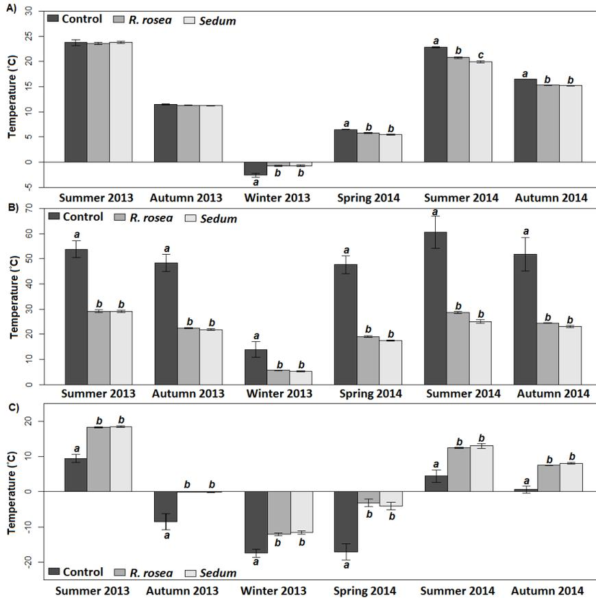
**Figure 5.** Substrate temperature (°C) at the SMU green roof depicting the average (A), maximum (B), and minimum (C) substrate temperatures for the conventional roof control, the *R. rosea* treatment, and the *Sedum* treatment. Those bars that share a letter are not significantly different (within the same season).
